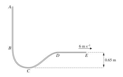
A smooth narrow tube AE has two straight parts, AB and DE, and a curved part BCD. The part AB is vertical with A above B, and DE is horizontal. C is the lowest point of the tube and is 0.65 m below the level of DE. A particle is released from rest at A and travels through the tube, leaving it at E with speed 6 m s<sup>-1</sup> (see diagram). Find
